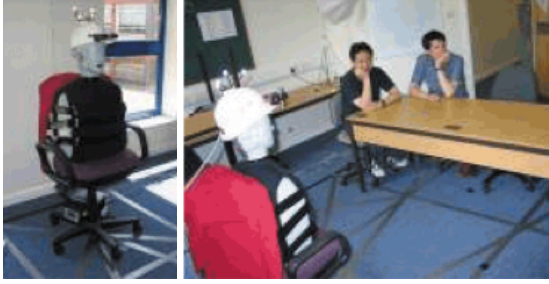
Fig. 1. This figure shows the mannequin used in our experiments as well as a typical setup. It is equipped with a binaural microphone pair and a camera binocular pair. When the mannequin is moved around, the position and orientation of its head are recorded as well.
