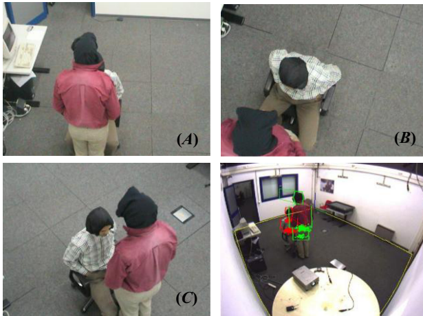
Fig. 11. Active views and tracker output during an occlusion. A predefined camera-to-target allocation may deliver (A), while the selection policy successfully allocated (C).
