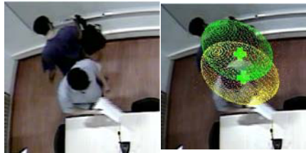
Fig. 1. Particles from the tracker A (yellow ellipsoid) falling into the exclusion zone of tracker B (green ellipsoid) will be penalized
